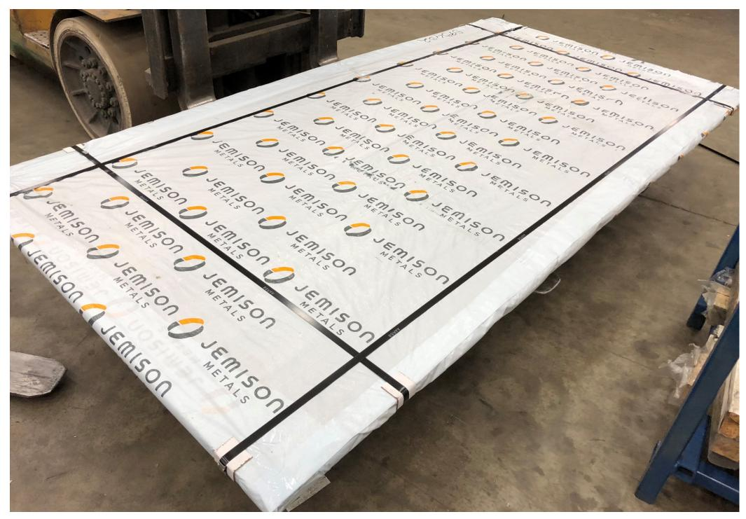
JD6, Full Paper Wrap, VCI bottom wrapped up, VCI top wrapped down & taped, Edge Protectors, 2 x Width & 2 x Length Bands
