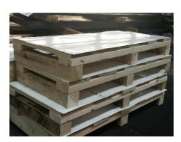
The skids are built the same just at different lengths for each part number (H04, H05, H09). Once we build a skid for the H12 I'll put the info together to send to sales to update the part spec.
